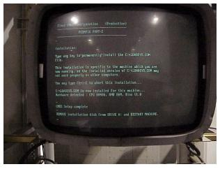
Remove the Final config disk from the A drive. Turn off the machine and wait 1 minute then turn the machine back on and when completed it should come up correctly.
